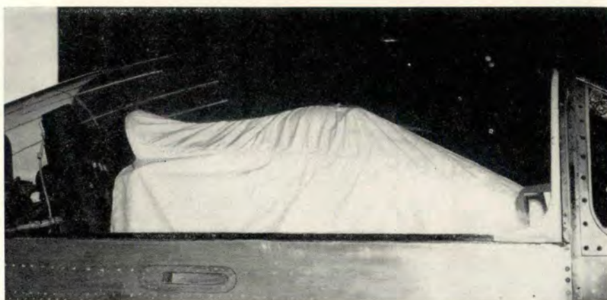
Utilizing a canopy style hood developed by Lt. Col. Frank J. Keller for the F-86A, the pilot in the above series of photos shows the ease of "going under" the new hood. Last photo shows the neat fit around the top of the instrument panel.
