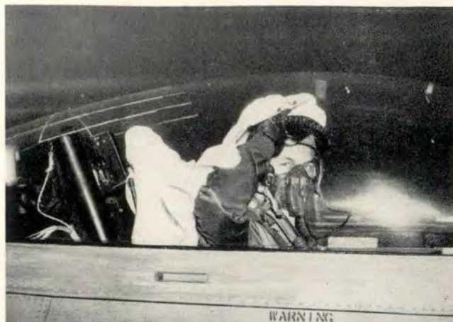
Utilizing a canopy style hood developed by Lt. Col. Frank J. Keller for the F-86A, the pilot in the above series of photos shows the ease of "going under" the new hood. Last photo shows the neat fit around the top of the instrument panel.
