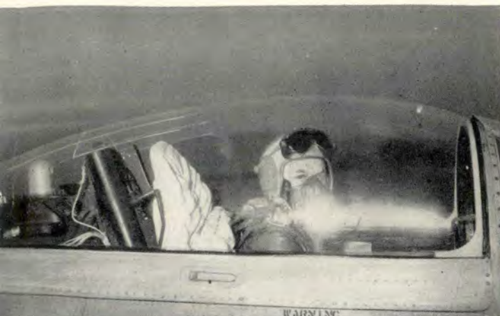
Utilizing a canopy style hood developed by Lt. Col. Frank J. Keller for the F-86A, the pilot in the above series of photos shows the ease of "going under" the new hood. Last photo shows the neat fit around the top of the instrument panel.
